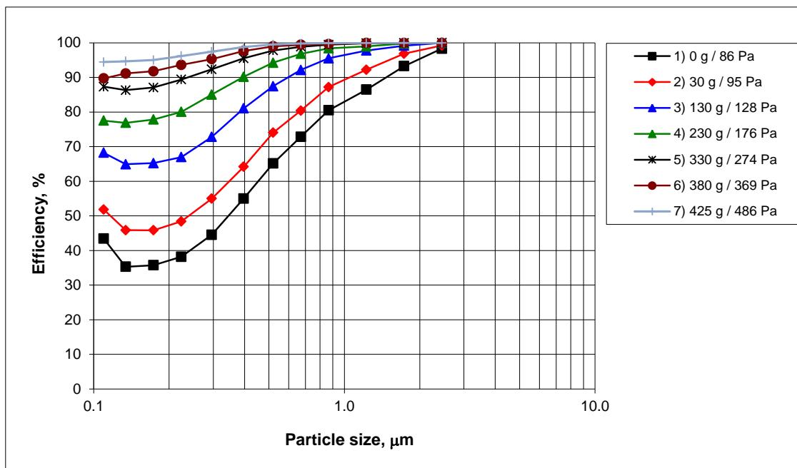
**EN779:2012 - Initial and average efficiency at different final test pressure drops**
